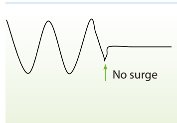
Waveform with the surge unit
