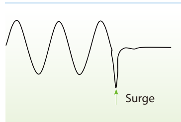
Waveform without the surge unit
