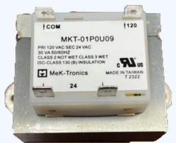
Mek-Tronics Class II transformers supply secondary voltages that are commonly utilized in various electronic, electro-magnetic and electrical control conditions. These include applications used with relays, solenoids, small motors, speed changers, pumps, heating elements, fans and blowers, electronic tubes, elevators, door openers and Thermostat control.
